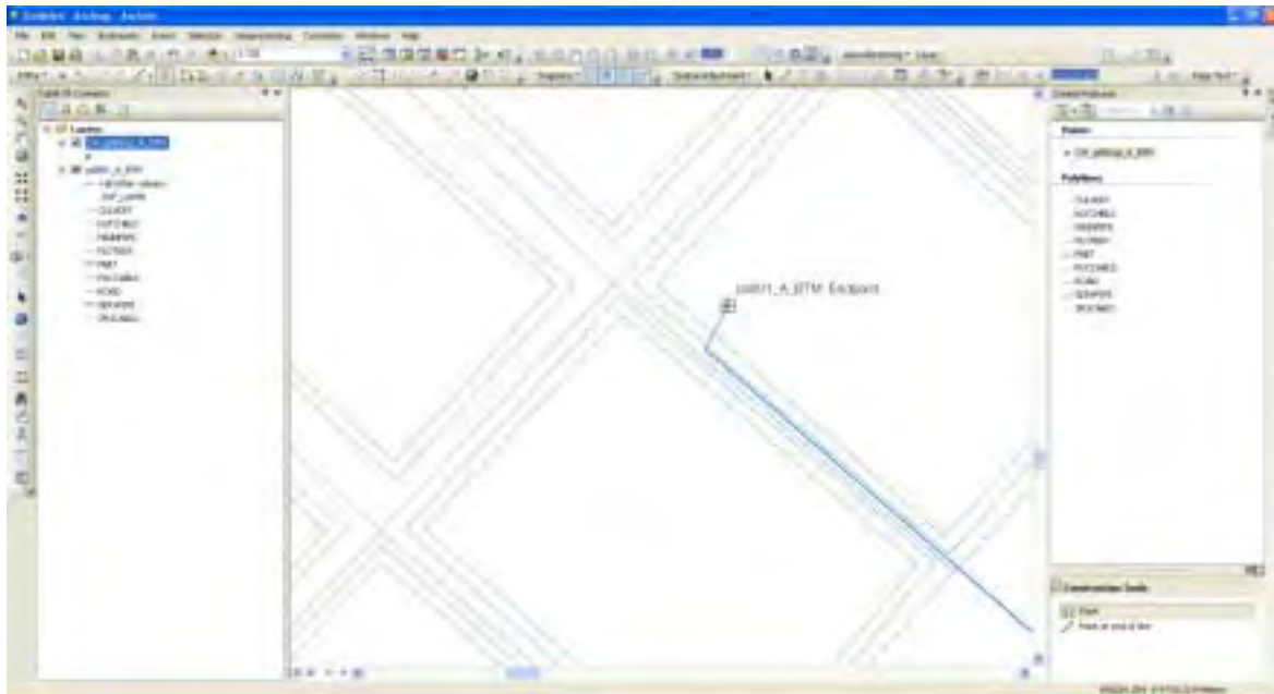
Figure 1.6: Adding service meter at the end of service pipe
