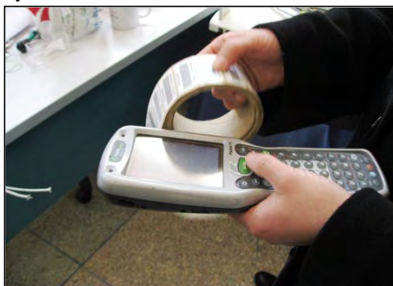
Picture 4: photo taken at Gharb- Chrarda- Béni Hssen Regional Maintenance Bureau. Equipment is registered with barcode system.
