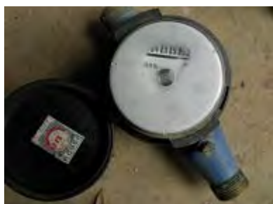
House water meter face blurred with CaCO 3 in Quang Son, Ninh Binh
