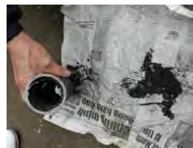
Water pipes with Manganese in Van Ha, Thanh Hoa (DN40mm)
