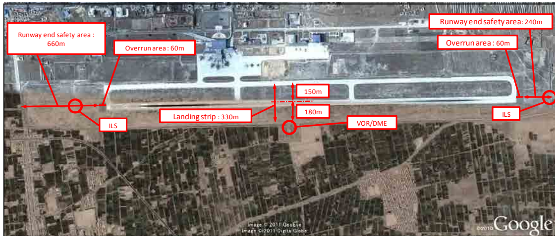
Figure-4 Status of Airport Facilities (created based on data from Google Earth)
