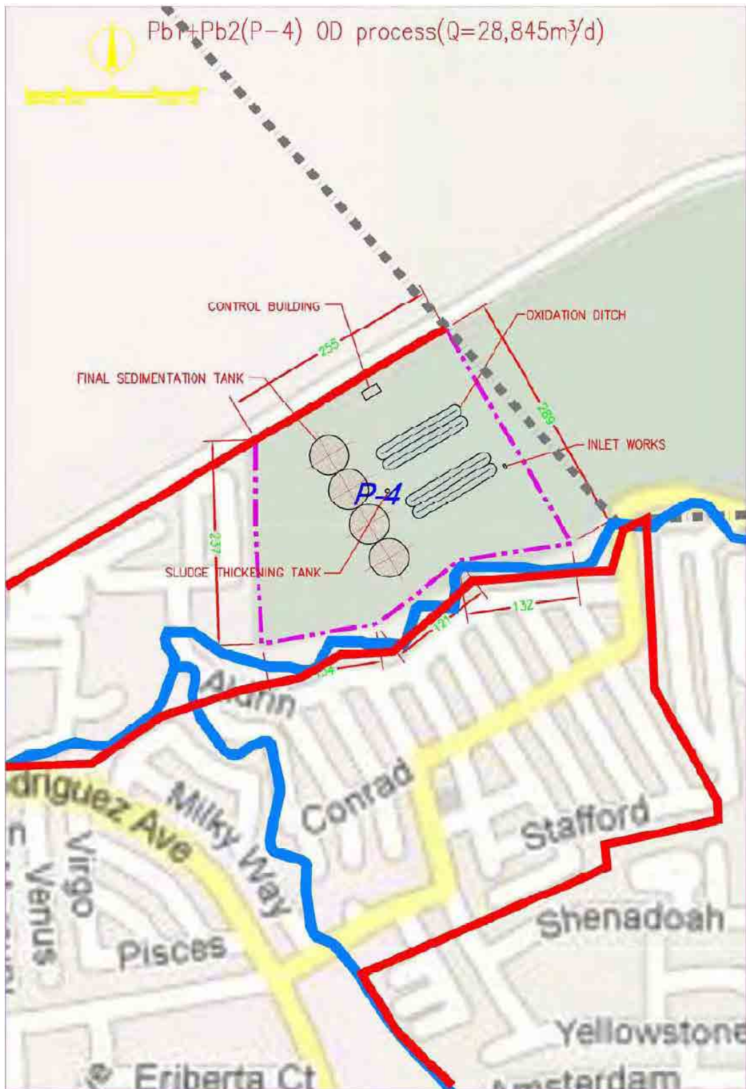
Figure 3.2-6 Pb1+Pb2 (P-4) OD (Q= 28,845m 3 /d)
