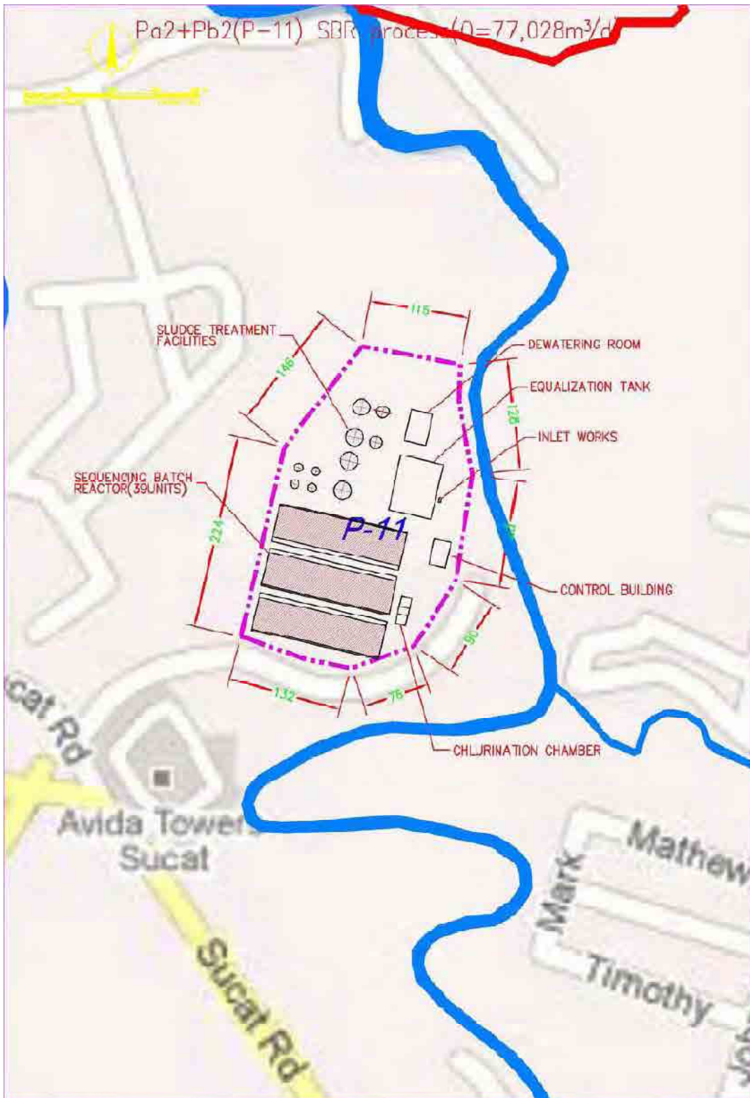
Figure 3.2-1 P2+Pb2 (P-11) SBR (Q= 77,028m 3 /d)
