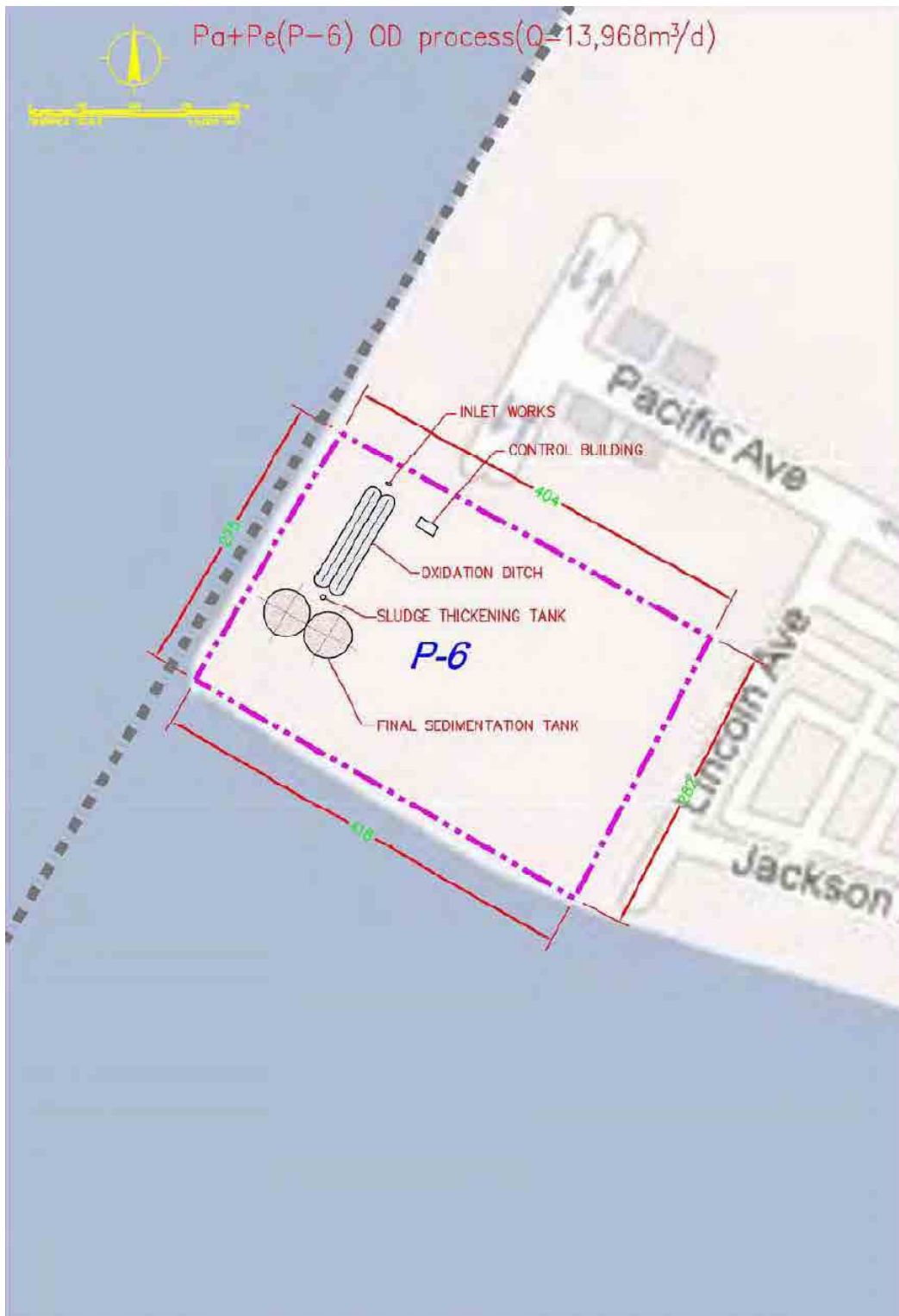
Figure 3.2-7 Pa+Pe (P-6) OD (Q= 13,968m 3 /d)
