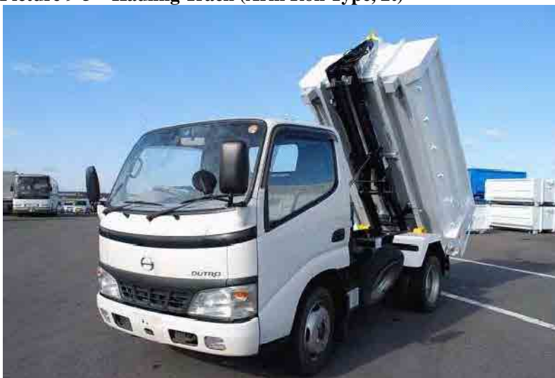
Picture 9-5 Hauling Truck (Arm Roll Type, 2t)
